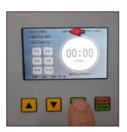
Once saved, the newly set voltage should appear on the Welcome screen when the unit is turned back on. This particular unit has been changed to 220V.
