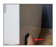
In engineering mode (voltage appears in the top, middle of screen), change voltage by pressing the 'P' button. Please wait until you see that the voltage has changed. Continue to press the "P" button until your country specific voltage rating appears.
